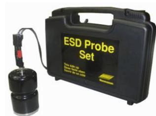
The Concentric Ring Probe can measure the volume resistance of planar materials using a flat conductive metal plate (not included). The Concentric Ring Probe may be used for the resistance measurements of ESD packaging including static shielding and other bags. Accuracy determined by the equipment used to take the reading. HP4339B used for this purpose.
