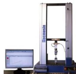
information at the touch of a button. Tests which can be provided include, but are not limited to, lap shear tests, friction tests, peel tests, three point bend tests, etc.
