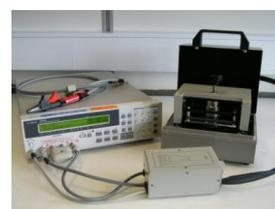
It is designed to reliably and repeatedly test solid parts. It can accommodate flat thin sheets ranging in size from 50 × 50 mm up to 100 × 100 mm. 28 and 50 mm diameter electrodes are available for testing.
