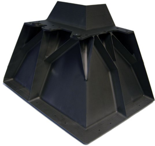
SolarBlack on Solar Orbiter component
