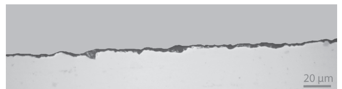
Hydroxyapatite coating on nitinol plate
