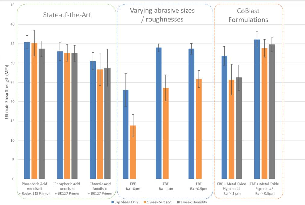
Of these, FBE- fusion bonded epoxy (thermoset polymer powder) has shown significant promise. Partially cured epoxy is deposited and co-cured with the adhesive. This promotes strong cross-linking and high strength, matching current state-of-the-art. Latest work has focused on the inclusion of corrosion-inhibiting pigments to improve strength retention after humidity and salt fog exposure.
