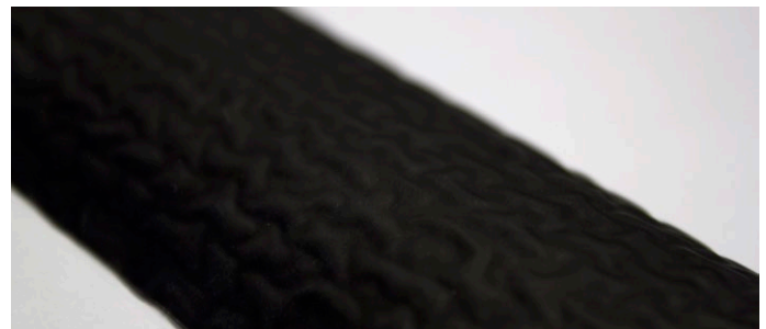
SolarBlack on 50 micron titanium foil
